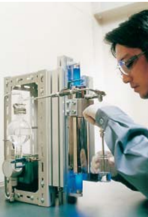
Dioxin decomposition experiment using fibrous photocatalyst
