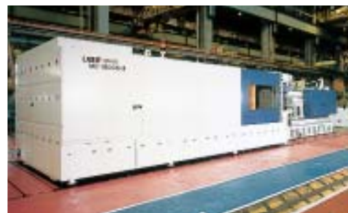
All-electric injection-molding machine with the world's largest clamping force—1,800 tons
