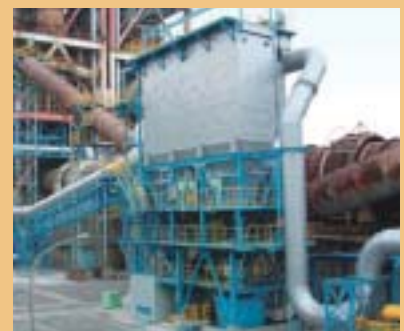
This facility uses a chlorine bypass system, achieving a high bypass ratio
