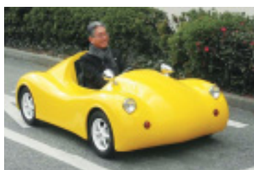
A minicar powered by lithium-ion batteries
