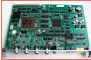
◀ A printed circuit board made using lead-free solder
